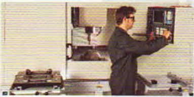
Machine in cutting cycle while second pallet is in position for reloading
