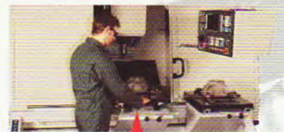
Return loaded pallet to machine cutting position
